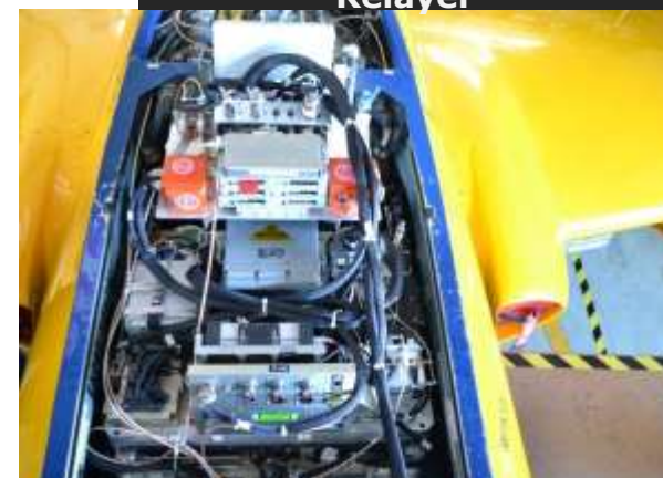
TMAC fitted into aft seat position
