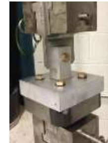
tension pull test to validate batch
