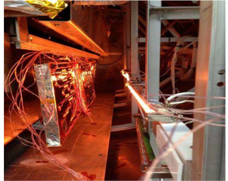
Fig. 3. Solar array wire coupons being heated in the V3 thermal cycle chamber. Samples are translated between the heated zone at the bottom of the chamber and the cold zone at the top of the chamber.
