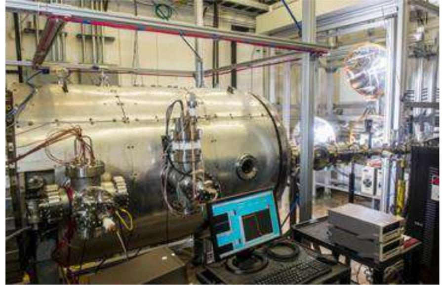
Fig. 4. HISET facility at MSFC. The facility is equipped with both broad beam and narrow beam electron and ion sources, as well as high intensity solar simulator lamps.
