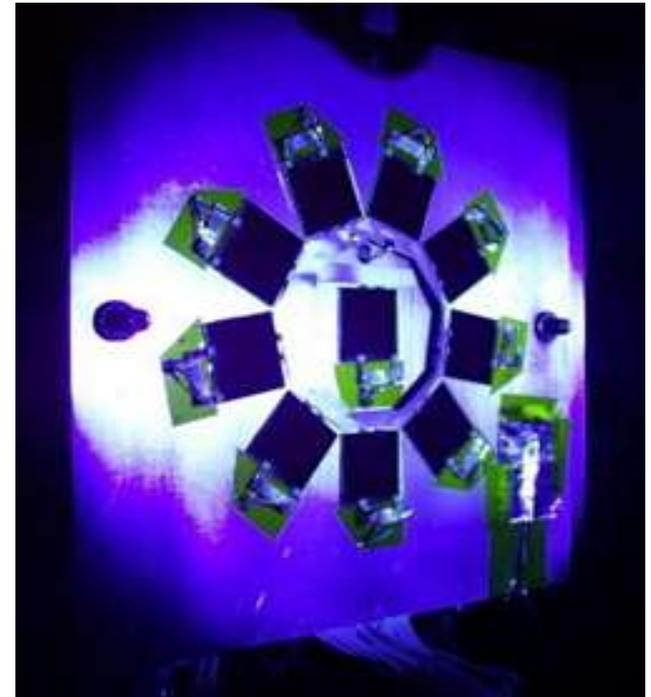
Fig. 1. Solar cell samples undergoing combined ultraviolet radiation exposure tests (VUV and NUV).
