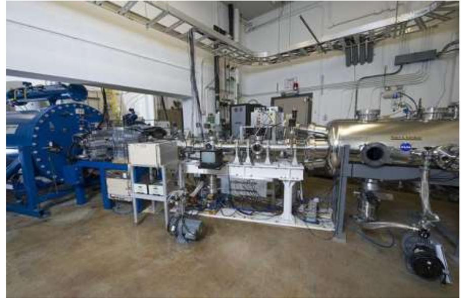
Fig. 2. The High Energy Charged Particle Radiation facility. The electron accelerator is visible on the left side (blue chamber) and the sample chamber is visible on the right side (silver chamber). The proton accelerator is not visible in this picture.
