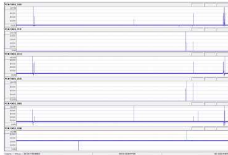
Transmitter data with –STC
