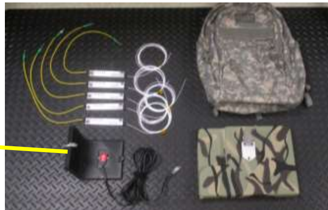
Box containing the sensors has an inertial measurement unit (IMU) to account for rotation of the subject in the global coordinate frame
