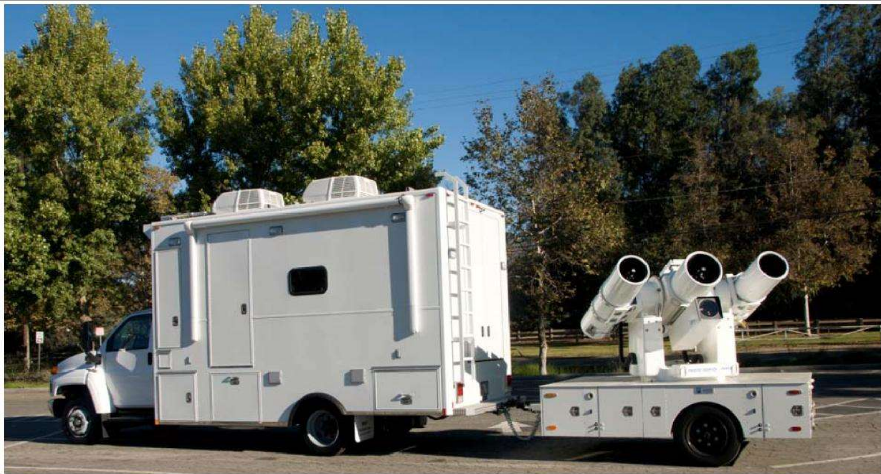
MMTS Control Van With Pedestal
