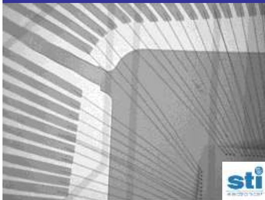
Damage to bond wires due to over voltage/current
