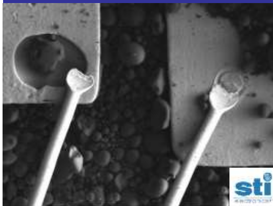
Damage to wire-bonds due to vibration or acceleration
