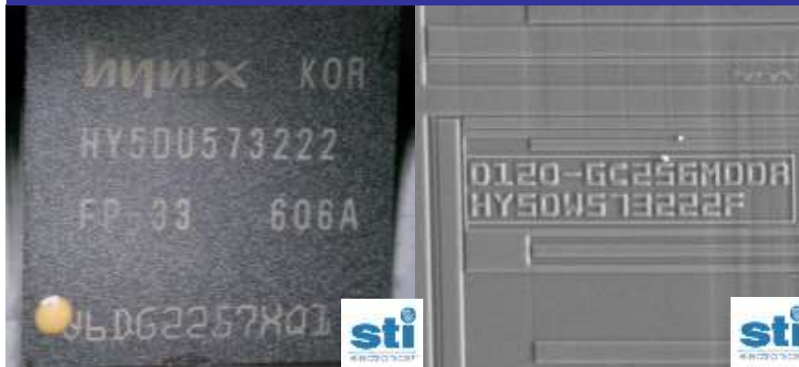
Counterfeit Parts - Die does not match the component markings
