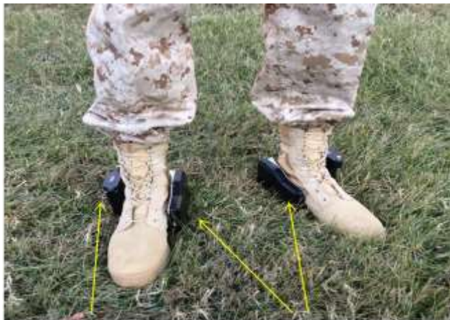
Battery enclosure Sensor package
