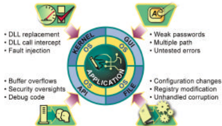
Figure 3. Applications surrounded by operating systems, and subsequently by the GUI, APIs, files and kernels, can be attacked on or from any of the many layers.
