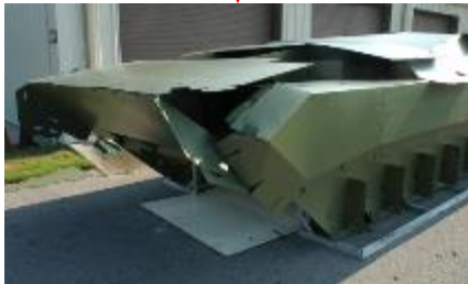
Target Outer Skin Installation
