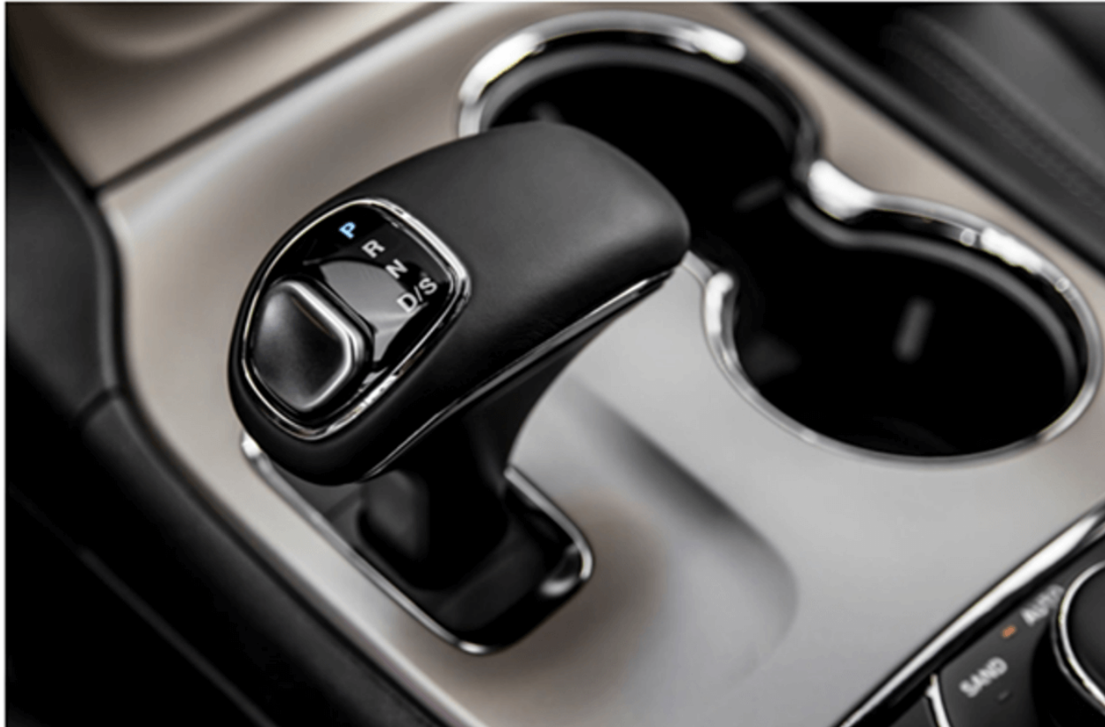
Figure 3: Monostable electronic (shift by wire) gearshift 2014-15 Grand Cherokee; 2012-14 Charger & 300 w/3.6L engine
