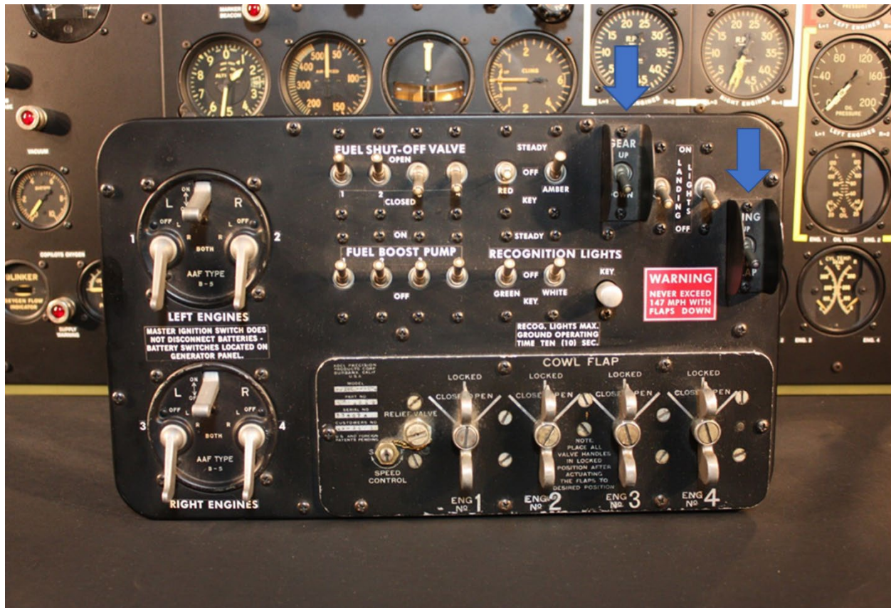
Figure 2: B-17 cockpit control switches for Landing Gear and Wing Flaps (note the arrows point to the identical switches for the landing gear (top row) and the wing flaps (second row) ( https://medium.com/swlh/the-flying-fortress-fatal-flaw-694523359eb )
