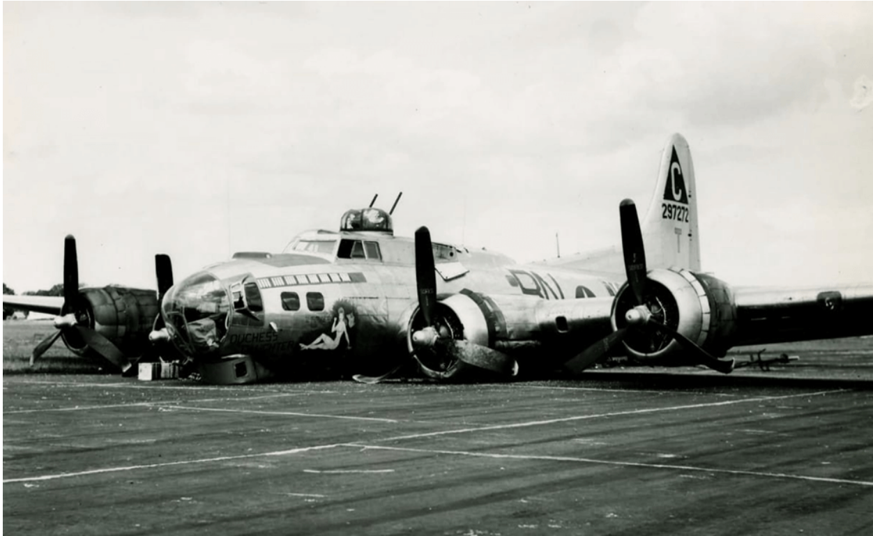
Figure 1: Result of a wheels up landing of a B-17 during World War II operations
