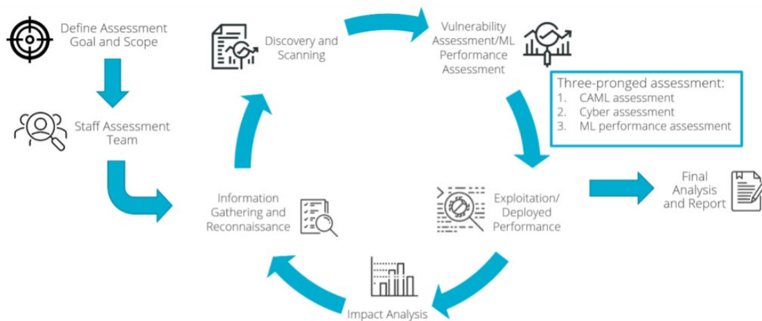
Figure 1: Overview of the methodology for assessing systems with an ML component. The key component is a three-pronged assessment: (1) an assessment of the ML component(s) to attacks that cause a failure or leak of unintended information; (2) an assessment of the infrastructure supporting the ML component(s) and how it may affect the performance of the ML component; and (3) an assessment of the performance of the ML component in contested environments.
